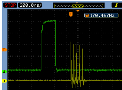
Fig. 16 Envelope SYNC vs. laser output
